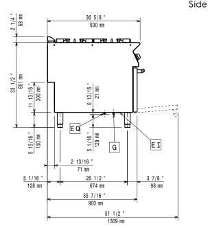
Electrical inlet (power) Gas connection
